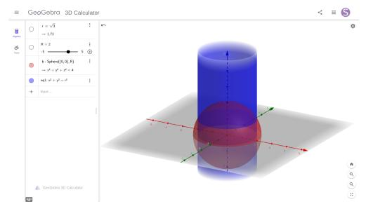
**Solution.** Required volume = Volume of the sphere - Volume generated by revolving the shaded region around the y-axis.
